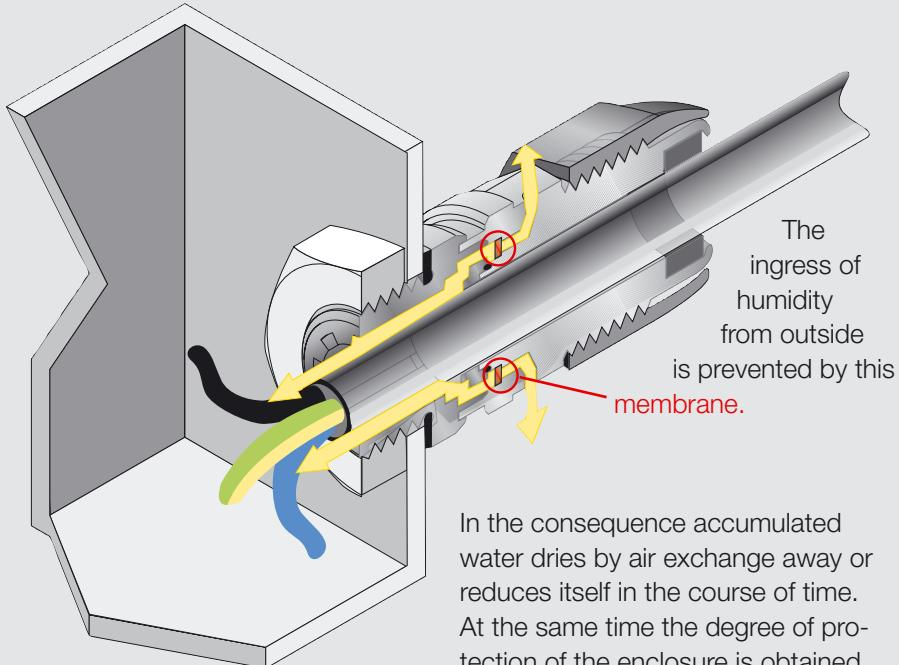
In the consequence accumulated water dries by air exchange away or reduces itself in the course of time. At the same time the degree of protection of the enclosure is obtained (up to IP 67)!
