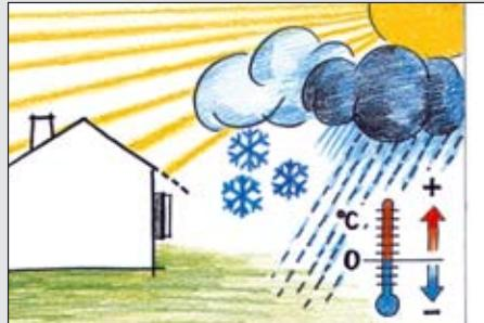
Condensation forms particularly in areas where large temperature fluctuations are expected, (= 'sweating' enclosures): e.g. with protected outdoor installations or unprotected outdoor installations.
