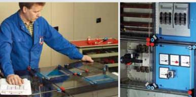
Individual box with electrical functions ...... can be built individually by the electrician for a distribution board.
