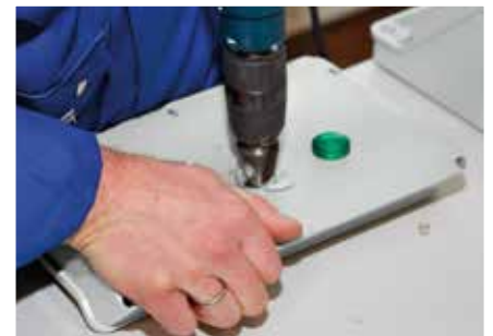
Pre-drill device cutouts or saw off with a jigsaw, depending on the shape.
