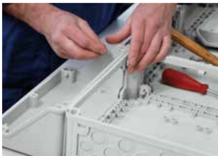
Assembly of the base of a Connection Box to Mi distribution boards via wedge connections
